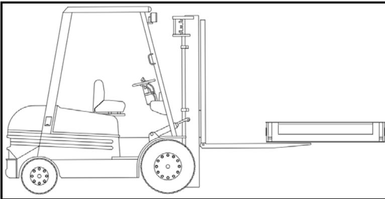
INCORRECT position of the module (bridge) on the forklift truck during the handling procedures.
