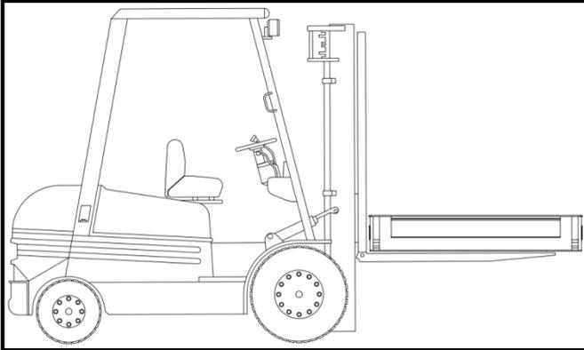
CORRECT position of the module (bridge) on the forklift truck during the handling procedures.
