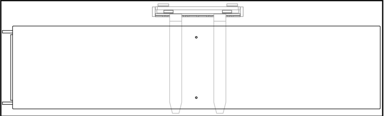
INCORRECT position of the module (bridge) on the forklift truck during the handling procedures.
