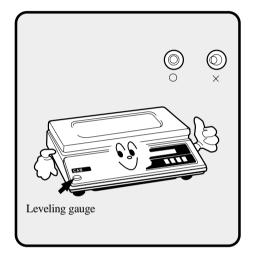
■ If the scale is not properly leveled, please adjust the 4 legs at the bottom of the scale (turn legs clockwise or counterclockwise) so as to center the bubble of the leveling gauge inside the indicated circle.
