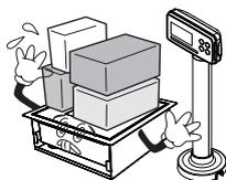
**Scale must be grounded to minimize electricity static.**
