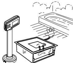
**Avoid placing the scale near heater or in direct sunlight.**
