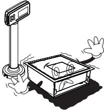
By adjusting 4 comers of the scale, set the scale even using the built in scale leveling indicator.
