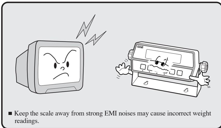
■ Keep the scale away from strong EMI noises may cause incorrect weight readings.
